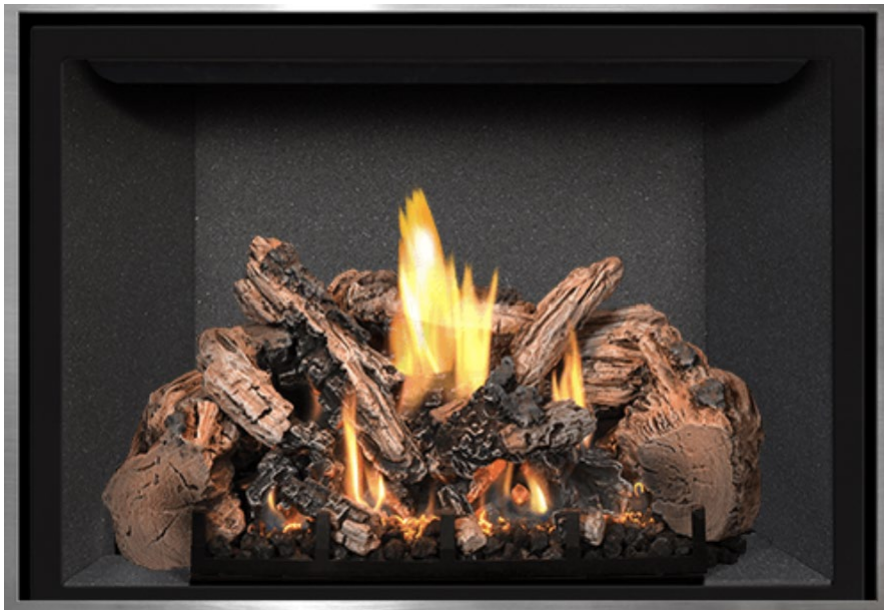
Figure 6-2 Burner Flame Heights: This image provides a visual reference for the burner flames burning at maximum height after the burners have been operating for 30 minutes or longer. A normal rear flame will be 1 to 2 inches above the rear log top edge. This, however, is dependent on the gas type, air shutter opening setting and vent system configuration. Actual flame heights can be slightly higher or lower when compared to this reference image.
